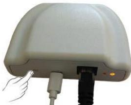
**4.2** With the hub in discovery mode, press the **Ok/Mode** button on the heater for 3 seconds until the Link symbol is shown.
