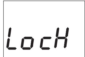
To unlock the keyboard, press the “+” and “-” buttons simultaneously for 3 seconds.
