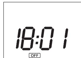
**3.6.2** If the heater is turned off via the main switch at the back of the heater or if the power to the heater is removed and the heater is not connected to a Wifi G- Control Hub then the time setting within the heater will be lost.
