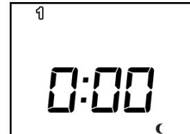
**3.2.4** Now the minutes start to flash. Press the "+" and "-" button until you reach the correct time (minutes) and Press the **OK/Mode** button.
